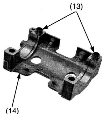
(13) dowel pins (14) camshaft holder
