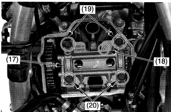
(17) camshaft holder (19) camshaft holder bolts (long)
